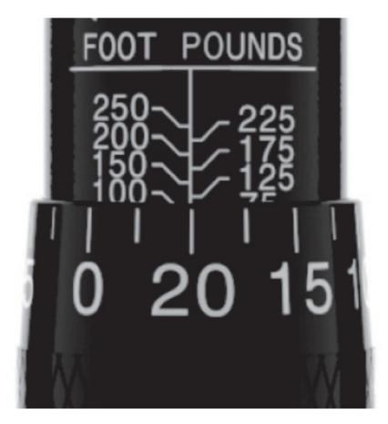
4. Lock torque setting by turning the lock nut clockwise until snug. The wrench is now set to measure 120 ft.-lb. of torque and ready to use.
