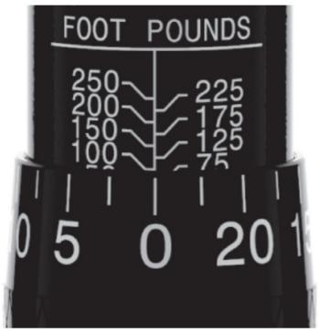
3. The micrometer-scale divides the main scale markings into 25 divisions. Every micrometer-scale marking equals 5 ft.-lb. To increase torque from 100 to 120, turn the micrometer handles clockwise until the "20" mark is centered on the vertical line of the main scale. 100 ft.-lb. (main scale) + 20 ft.-lb. (micrometer scale) = 120 ft.-lb.
