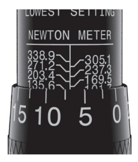
To increase torque from 135.6 Nm to 145.0 Nm, turn the micrometer handle clockwise until the "7" mark is centered on the vertical line of the main scale. 145.0 Nm = 9.4 Nm = 9.4 Nm = 9.4 Nm = 7 micrometer-scale markings. The wrench is now set to measure  $145.0 \text{ Nm} = 135.6 \text{ Nm} = 9.4 \text{ Nm$
