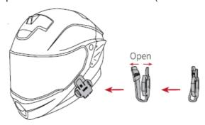
2. Install by 3M Tape mounting bracket: Except for using the clamp mounting bracket, you can also use the 3M mounting bracket instead. First, tear off the protective paper on the back of the 3M tape, then stick the 3M mounting bracket to a suitable position on the left side of the helmet. Press for 15 seconds to allow the glue 24 hours to dry.(As shown on the left).
