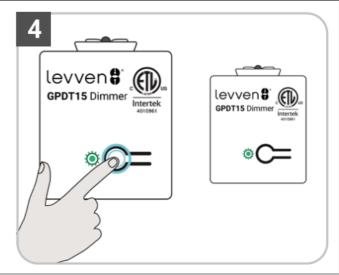
Both LEDs on each controller will start blinking red and green to confirm a signal is received.
