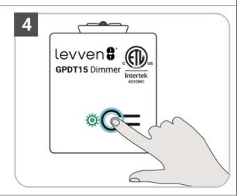
The LED on the controller will start blinking red and gr een to confirm a signal is received. Press and release the pair button on the controller aga in to complete the pairing. Its LED will flash green 3 tim es to confirm pairing.
