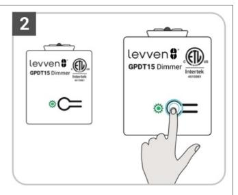
Press and release the pair button on the first controller to initiate grouping. This controller's LED will blink gree n.
