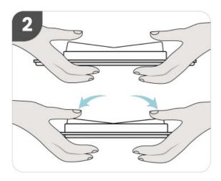
**Squeeze and release both ends of the switch simultaneously.** Both ends MUST be pressed at the same time to send the pairing signal to the power controller.
