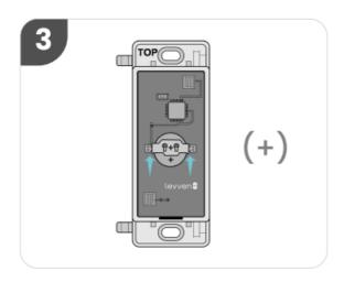
Replace a new battery by pushing it from the bottom of the holder, with the positive (+) symbol facing out. Use ONLY a CR2032 3V 225 mAh lithium coin cell battery.
