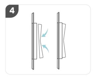
Snap the rocker back into the switch by pressing the rocker hinge into the switch body.
