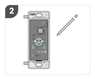
Use a toothpick or similar item to push the battery out of the holder from the top of the holder. Handle the battery as per instructions provided in Important Notes.
