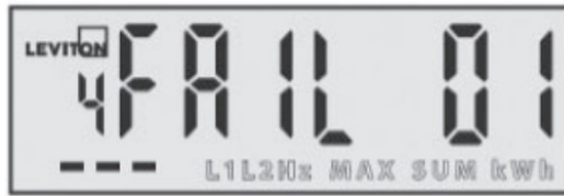
Error Screen Showing a Failure code, Factory Service Required
