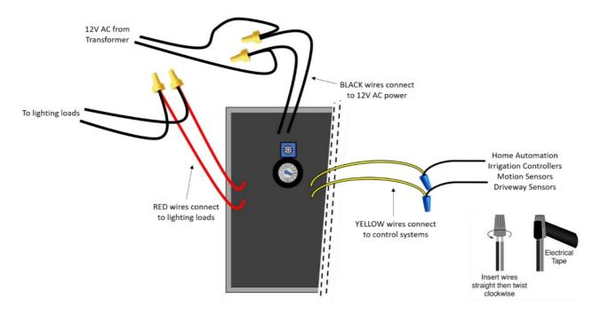
**NOTE:** Multiple zones may share the same power source, but never connect red wires in parallel as each output circuit must remain independent. When connecting more than 2 wires be careful to use the correct size wire nut. Yellow wire nuts are provided for the larger wires and blue are provided for the smaller control wires. Please refer to wire nut sizing charts when connecting multiple wires. The yellow wire nuts provided have a maximum capacity of (3) 12ga wires.
