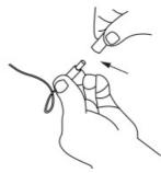
4. Put the AAA battery into the remote control.
