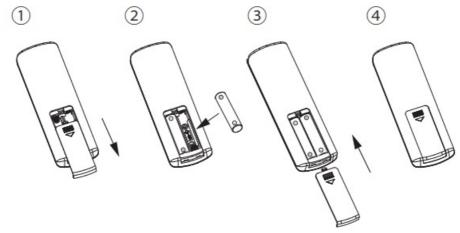
5. Put the 27A battery into the wireless wall switch.
