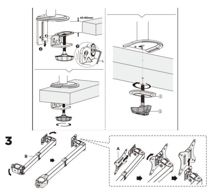
You will need to position the VESA Mounts to an UP position. To do that insert the VESA plate and rotate it to an upright position as shown. When complete, remove the VESA plate and proceed to the next step.
