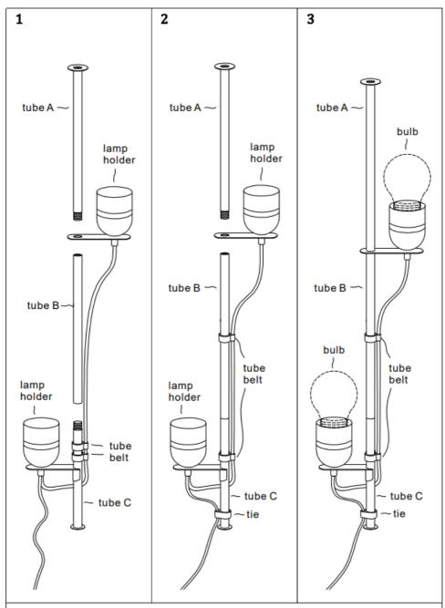
Tips: To avoid bending during installation, please ensure that the connection between the tubes is correct and tightened tightly.
