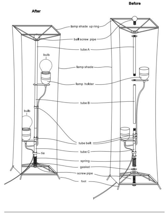
PLS assemble the lamp step by step according to the installation diagram(figure1~figure15)
