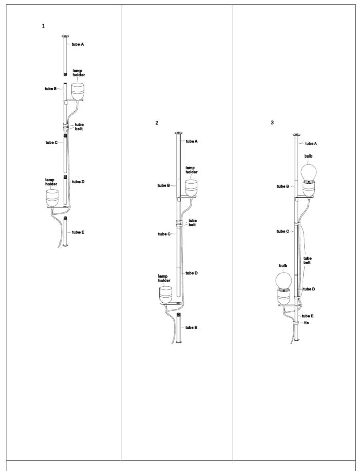
Tips: To avoid bending during installation, please ensure that the connection between the tubes is correct and ti ghtened tightly.
