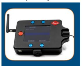
6. Select "Scan WL" by pressing the blue button on the lower left side of the remote. Once pressed, any powered on receivers should appear on screen. Once you've identified which receiver you would like to pair, scroll to it.
