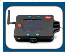
7. Press the knob once to select the receiver and once more when you would like to connect. You'll know you're ready to pair by the blinking red and blue lights. If there was an interruption in the pairing process and the lights stopped blinking, simply select "IDENT" and resume the pairing process. The LED lights should blink while connecting and then stop when successfully paired.
