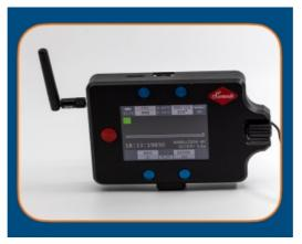
9. When ready to record, press the red button. This brings up your record menu and begins the recording process. If using camera memory, a red line will progress across the screen while recording is in progress.
