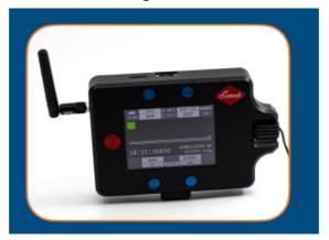
11. If you're looking for additional menu options, press both blue buttons on the bottom of your Semote from the control screen.
