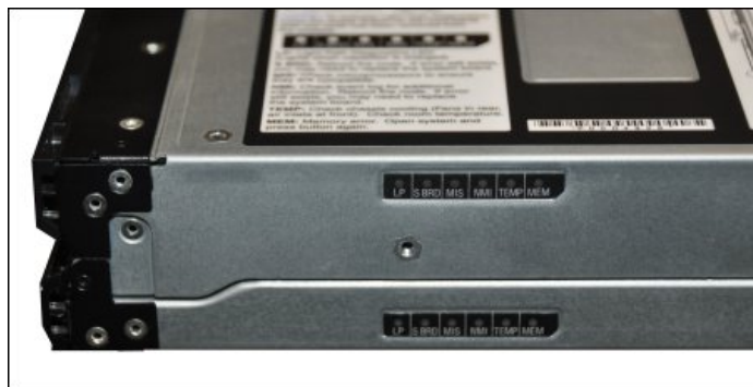
Figure 10. Location of x222 light path diagnostics panels To illuminate the light path diagnostics LEDs, power off the server, slide it out of the chassis, and press the power button. The power button doubles as the light path diagnostics remind button when the server is removed from the chassis.
