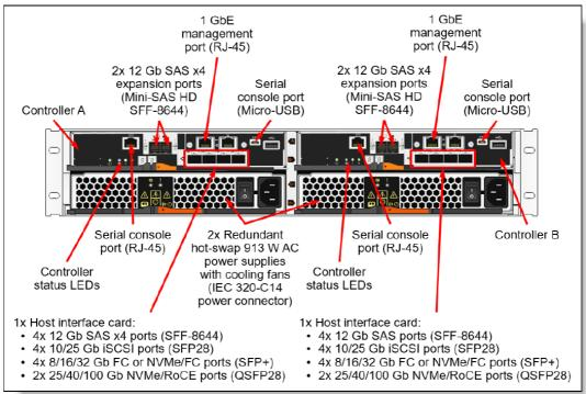
The rear of the ThinkSystem DE6000F 2U SFF controller enclosure includes the following components:
