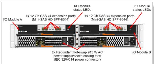
The rear of the ThinkSystem DE240S 2U SFF expansion enclosure includes the following components:
