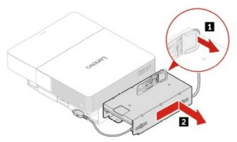
Note: Hold the latch in step 1 when removing the power adapter cage.
