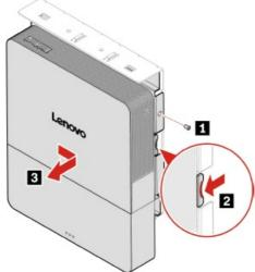
Note: Hold the latch in step 2 when removing the top bracket.
