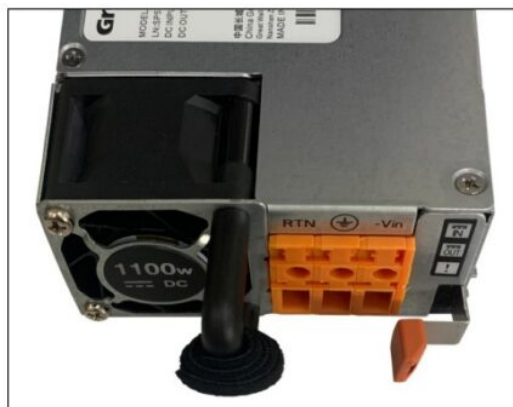
Figure 14. Connector on the ThinkSystem 1100W -48V DC Hot-Swap Gen2 Power Supply
