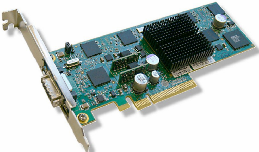
Figure 3. Chelsio S310E Single-port 10GbE PCIe x8 Adapter (CX4 connector), 46M1813
