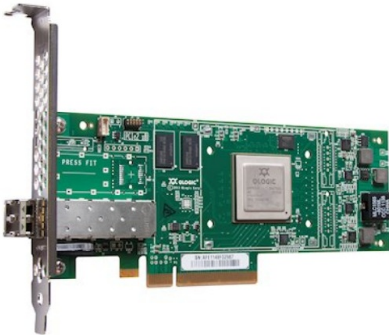
Figure 2. QLogic 16 Gb FC Single-port HBA
