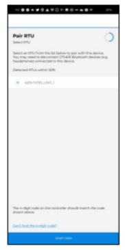
2. Select the Proper RTU in the list shown to complete pairing to your device.
