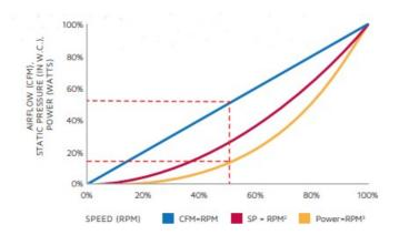
Based on the theory of Fan Laws, the blower operates at full power when it is running at full speed, but the same fan running at 50% speed consumes only 12.5% of the rated horsepower. By reducing airflow by half, the horsepower consumption is reduced by 87.5%, resulting in significant energy savings.
