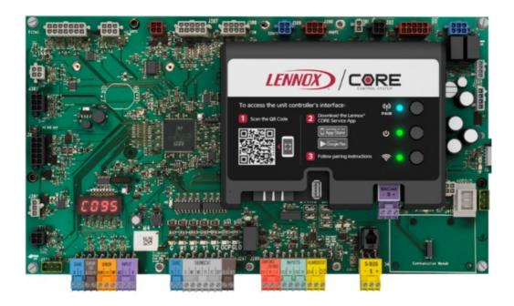
The Lennox CORE Lite Controller provides built-in S-BUS support for simple connection to the Lennox Comfort Sense family, such as the CS8500. Optional BACnet MS/TP modules support all existing objects from the Lennox CORE Controller and legacy Lennox control devices.
