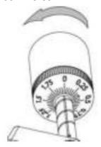
**NOTE:** The recommended down force for the factory fitted cartridge is 3.0±0.5g.
