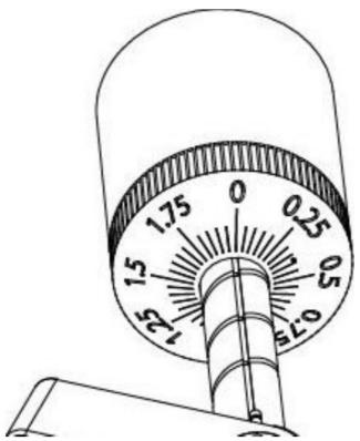
• Rotate the counterweight counter clockwise (seen from the front) to adjust the down force according to the cartridge manufacturer's recommendations. One mark on the scale represents 0.05g of down force.
