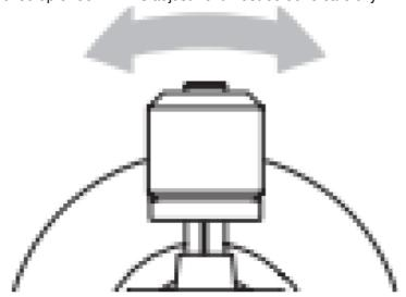
• Once the tonearm is correctly balanced return it to its' rest. Hold the Counterweight without moving it, and gently rotate the Down force Scale ring until the zero is in line with black line on the rear of the tonearm. Check whether the arm still balances out.
