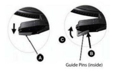
2. Push the needle headshell upwards in the direction illustrated by "C" until the needle locks into the tip position.
