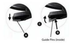
2. Push the needle head shell up wardsin the direction illustrated by "C"until the needle locks into the tip position.
