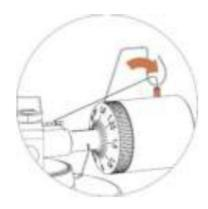
Slip the loop of the anti-skating weight's thread over the 3nd groove of the stub to set the correct anti-skating force for the factory-fitted cartridge. Feed the thread through the loop of the wire support.
