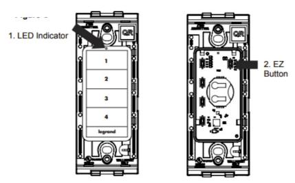
Reset To Factory Default Deleting a device from the app will reset it to factory defaults. To manually reset the device to factory defaults press and hold the EZ button for 10 seconds until you see the LED blink red then release. The LED will change to solid red when the reset is complete
