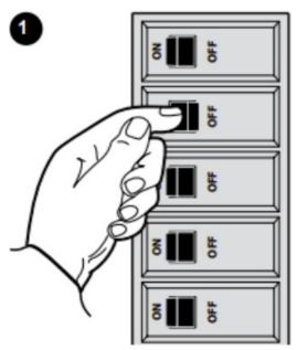
**NOTE**: Ensure power is off to all devices in electrical box.
