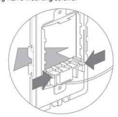
Remove spacers from the frame. Since this dimmer fills the frame completely, you will not need the spacers. From the back of the frame, pinch the tabs on the spacer to release.
