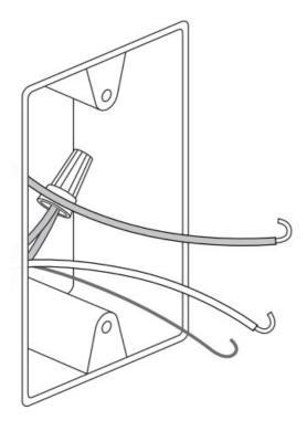
2. If necessary, cut wires and strip insulation using stripping guide on back of switch.
