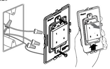
Remove the grounding wire label from the back of the device to access the ground wire. Connect it to the box ground using provided wire nut. Terminate and cap with wire nuts any] other wires in the box. Mount devise to wall box with screws provided. Tighten screws just enough to hold the frame in place. Do NOT overtighten.
