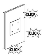
• There are three click-stops to adjust the fit of the wall plate to the device and the wall.
