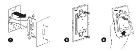
In case of multi-gang installation, replace the provided frame with adorne ™ multi-gang frame. While holding the frame with one hand, push the device up slightly until it snaps out and then pull it out of the frame. Secure the device to the multi-gang frame using frame mounting screws.
