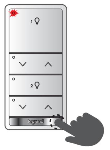
2. If the top button LED did not flash red, the configuration button is locked. Press-and-hold the configuration button and the top-most button on the switch simultaneously until the top button LED flashes red (approximately 3 seconds). This signals that the configuration button is unlocked.
