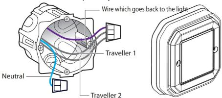
Use a connector to connect all 3 wires together (travellers 1 and 2 and lamp return wire). Use an other connector for neutral wire.
