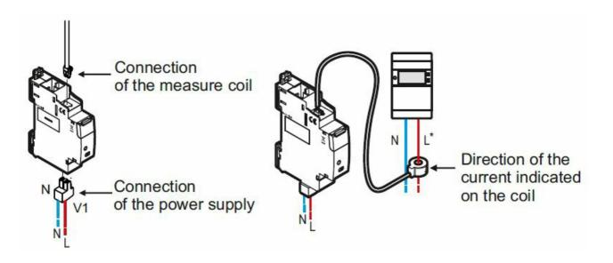
A circuit breaker with rated current C2 to C16 is necessary depending on wire section used for supplying the smart load shedder.
