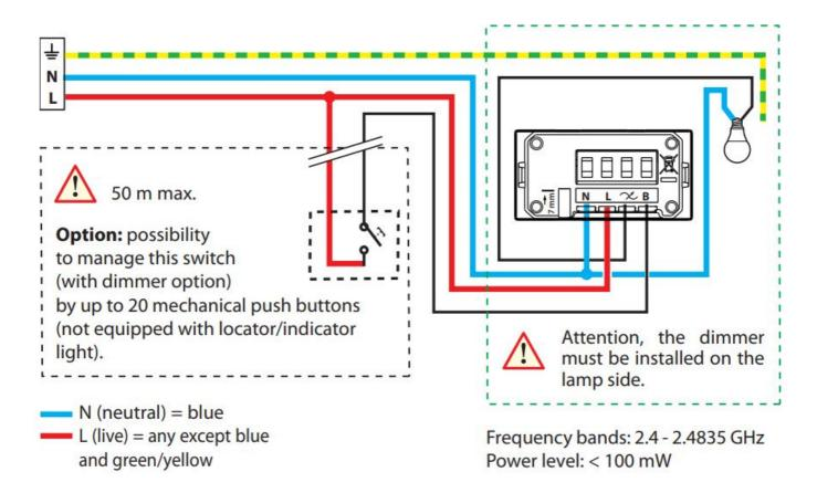
The connected switch with neutral (with dimmer option) works with standard or dimmable bulbs including LED. LED dimmable bulbs are mandatory for optimal dimmer usage.
