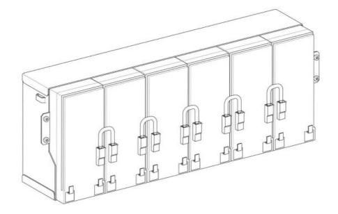
Keep the batteries firm to the block by fixing a metal bar with the four screws provided.
