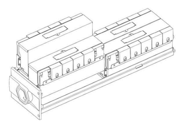
Connect in series the two new blocks to the ones already in the drawer using the cable provided and respecting the polarity (connect a positive terminal to a negative terminal). Connect the free terminals of the two batteries located close to the handle of the drawer to the cables that go to the back of the drawer. Check the correct polarity of the whole cabling.
