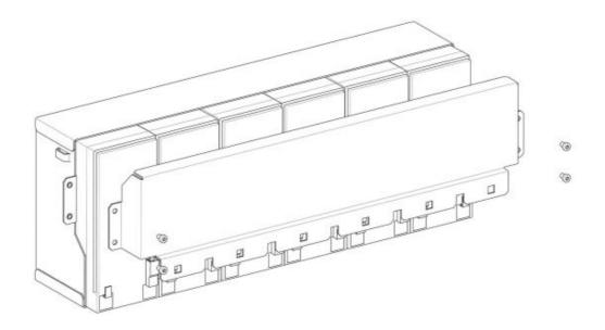
Insert the terminal covers on the four central batteries of the block but not on those at the extremes.
