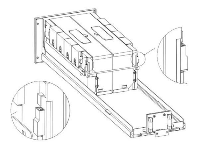
Once the connection is done, insert the terminal covers on the two batteries and push the blocks at the bottom of the drawer.
