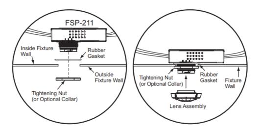
**NOTE:** The Outside Fixture Wall thickness should be no greater than 0.125" (3.18mm) for optimal sensor mounting and security.
