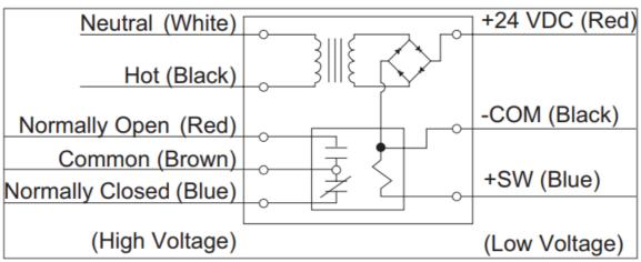
The power pack is attached to existing junction boxes. All low voltage wiring should be at least 22 gauge wire. All high voltage connections should be at least 14 gauge. Always check existing building codes. After initial wiring is complete, check to verify that power pack is wired correctly. Incorrect wiring can cause damage to power pack, lighting system, and occupancy sensor.
