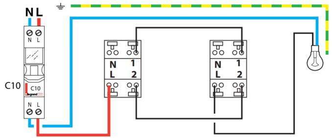
Replacement of an existing 2-way switch by a connected switch + wireless light switch Previous switch replaced by the wireless light switch
