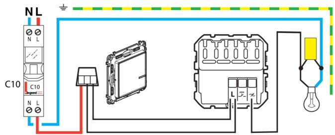
Use a connector to connect all 3 wires together (travellers 1 and 2 and lamp return wire). Use a dedicated connector to insulate the neutral wire (if present)
