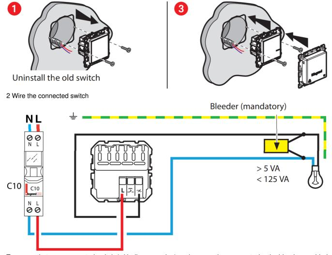
To ensure that your connected switch (with dimmer option) works correctly, you must wire the bleeder provided as close to the load as possible and put a bulb in before turning the power on.
