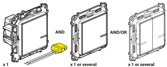
Connected switch without neutral (with dimmer option) + bleeder Wireless light switches for all other controls (not included in this pack)
