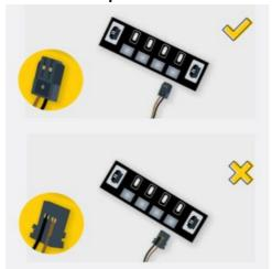
Take extra care when inserting the micro connectors to micro ports of Micro Expansion Boards. Connecting Micro Bit Lights to Micro Expansion Boards is similar to connecting lights and cables to Strip Lights. With the expansion board facing up, ensure the side of the connector with the wires exposed is facing down. If a plug won't fit easily into a port connector, do not force it. Use your fingernail to push the plastic part of the connector to the micro port.
