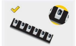
If you look carefully inside each of the ports, each port contains 2 small pins that should be straight. You will be able to identify a faulty port if it has any bent pins.
