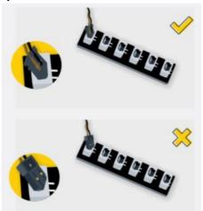
Take extra care when inserting connectors to ports of Expansion Boards. Connectors can be inserted only one way. With the expansion board facing up, look for the soldered "=" symbol on the left side of the port. The connector side with the wires exposed should be facing toward the soldered "=" symbol as you insert it into the port. If a plug won't fit easily into a port connector, do not force it.
