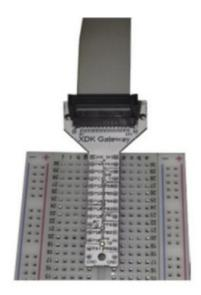
Connect the 26-pin cable which is included in delivery with the extension board to the 26-pin connector of the XDK 110. The extension board offers a simple way to implement additional functions. It is optimized for the use of breadboards.
