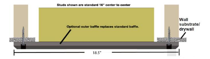
Pixel Pro can be ordered with an oversized outer baffle to allow for in-wall installation. The outer baffle is 18.75" long and 18.5" wide. Four mounting screws are to be installed through the center of the grille cups into the wall framing. Care should be taken to avoid electrical or plumbing- before cutting into the wall or installing screws into studs.
