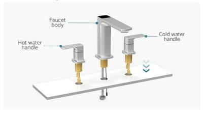
STEP 3: Install gaskets, nut and fasten the screws.
