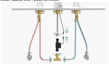
STEP 7: Turn the faucet on and check for leaks. (Do not turn the faucet on before the installation is complete)
