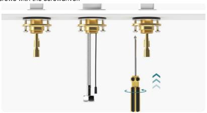
**STEP 5:** Connect the Hot and cold water lines, and tighten them clockwise.
