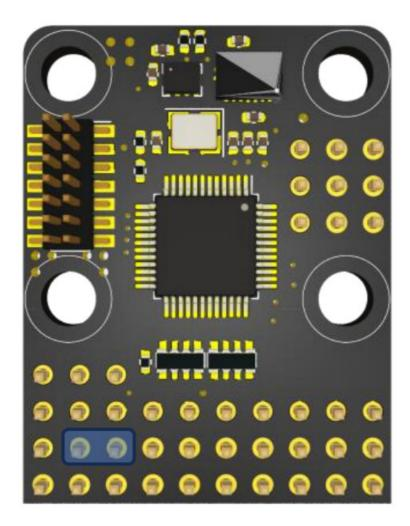
It's recommended to use the supplied 3300uF/16V capacitor to get a more stable and secure working voltage for the PMU. The capacitor can be plugged onto any one of the free input or output sockets of the FC.
