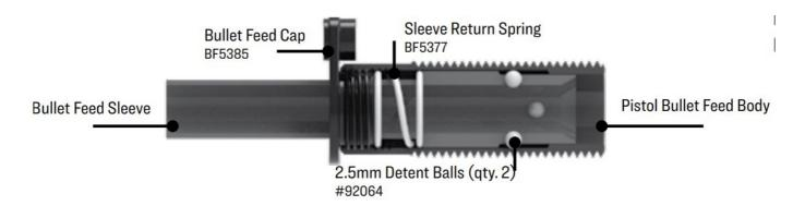
1. Measure projectile's cylindrical portion, "A" section. Refer to the bullet length chart (see reverse) to confirm the two detent balls are installed in correct holes of bullet feed sleeve. Detent balls are installed in upper holes from factory.
