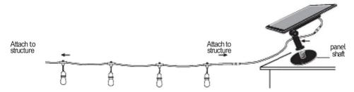
**NOTE:** Select a location with sunlight. Lights may turn on during the day if the solar panelis installed in a shaded area.
