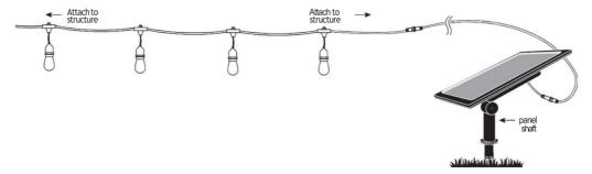
**NOTE:** Select a location with sunlight. Lights may turn on during the day if the solar panel is installed in a shaded area
