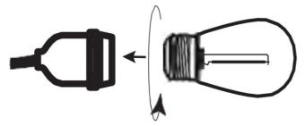
NOTE: LED bulbs provided with left handed thread base, Bulb will not screw into standard socket.
