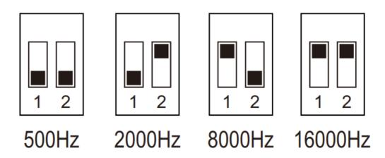
When power is off, select the DIP switch firstly, then press holds the MATCH key, and power up the controller at the same time, the RUN LED indicator will flash white color two times means the PWM frequency setting is successful. We can select four PWM frequencies: 500Hz, 2000Hz, 8000Hz, or 16000Hz. Higher PWM frequency will cause lower output current, and higher power noise, but more suitable for the camera(No flickers for video).
