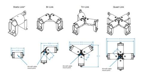
\*Static links apply to continuous runs only; all other links apply to patterns/shapes.
