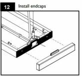
Insert the foam gasket onto the fixture end and ensure the gasket is firmly seated inside the housing. Using supplied Phillip screws, snug the endcap in place. Align the endcap to fixture housing before final tightening. Cut excess suspension cable if necessary.
