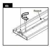
Twist the screwdriver and the tab on the access panel will POP UP. Repeat steps 4 at the other tab on the access panel.
