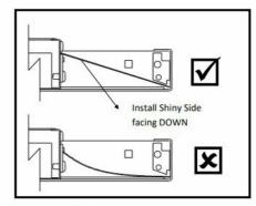
Re-install the upper diffuser (SHINY SIDE facing DOWN). If applicable, install optional 75 or 100% downlight reflectors on top of upper diffuser in correct orientation.
