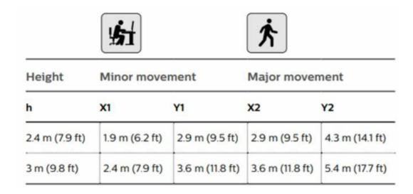
The detection area for the movement sensor can be roughly divided into two parts;
