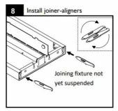
Prepare the joining fixture by twisting apart the joiner pair and inserting into crossplate (DO NOT INSERT INTO THE FIXTURE ALREADY SUSPENDED). Open the wire access panel of the joining fixture.
