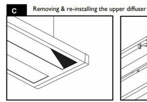
If the fixture is mis-handled during installation, a shadow may appear in the luminous window. This is caused by the upper diffuser being pushed below the LED.
