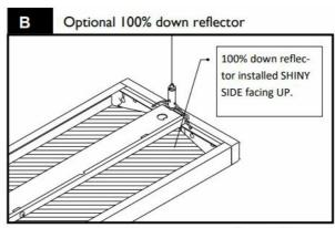
FloatPlane Fixtures available with a factory installed, solid 100% down reflector (shown as hatched lines). For best optical performance, reflector must be installed SHINY SIDE facing UP. Note the 100% down reflector is installed on top of clear acrylic upper diffuser.
