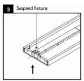
With 2 people, raise the fixture up to the suspension cables and feed through grippers. Set fixture to desired height.
