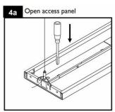
Identify power feed location on fixture. Insert a medium size flat blade screwdriver into slots on access panel.
