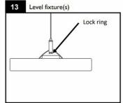
Loosen cable gripper lock ring, adjust sling mount(s) to level fixtures. Tighten lock ring when complete at all mount locations. Cut excess suspension cable if necessary.
