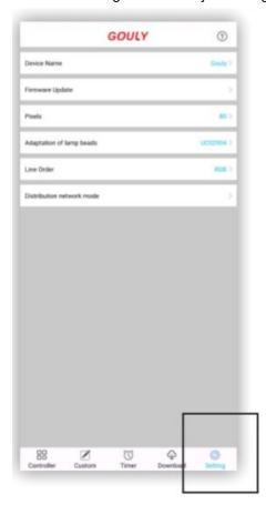
4. Select the number of pixels, chip type of digital light and Line Order. Use UCS2904 for LED World's digital lights and RGB as Line order. See the guide for pixel counting on the second page.
