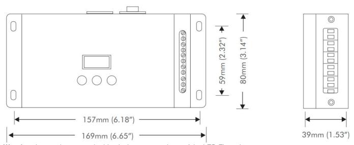
**Warning:** Input voltage must be identical to output voltage of the LED Fixture! WIRE 6-8 MM (0.25-0.30")
