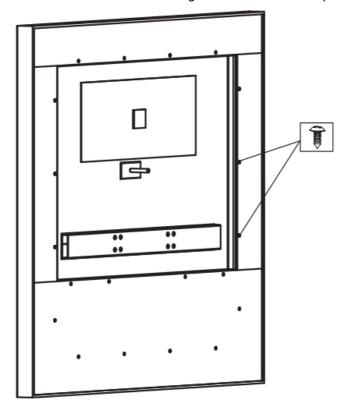
7. Remove the led strip cable from the terminal station and take out the LED strip.
