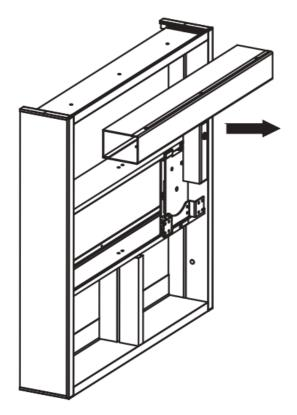
8. Unscrew both ends of the led driver cover.
