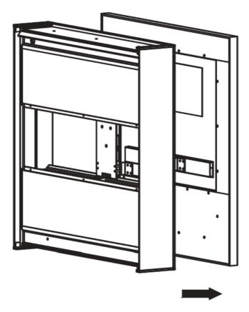
6. Remove the screw connecting the door to the back plate on the door, take out the back plate.
