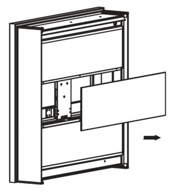
3. Remove the screw connecting the cabinet to the door.
