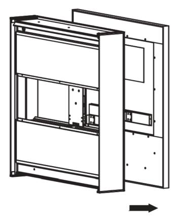
6. Remove the screw on electric ail box of the cabinet
