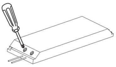
9. Remove the wires at both ends of the led driver, Unscrew the led driver base.
